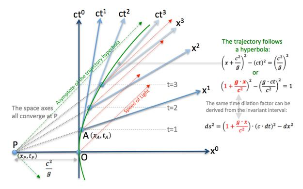
The position of each event along the world line of the accelerating spacecraft forms a hyperbola that passes through the origin. Its equation contains the time dilation factor. Note how the acceleration trajectory follows the hyperbolic shape of space-time.
